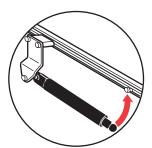
When tonno is removed, stow the gas shock against the shock hold down stud.
